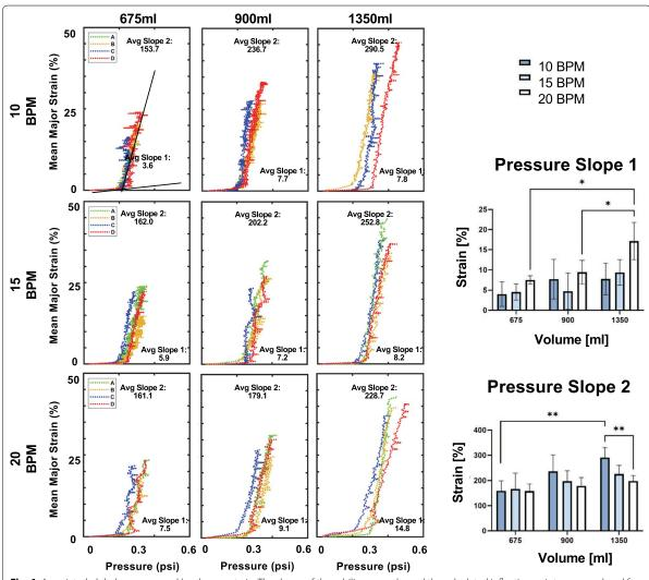
Fig. 6 Associated global pressures and local mean strain. The slopes of these bilinear graphs and the calculated inflection points were analyzed for statistical significance to assess local tissue compliancy
