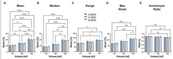
Fig. 4 Statistical analysis of mean (A), median (B), range (C), and maximum strains (D), and anisotropic ratios (E) for varying rates and inflation volumes. Significant volume dependency was observed for all data sets between 675 and 1350 ml, and no significant rate effects were found
